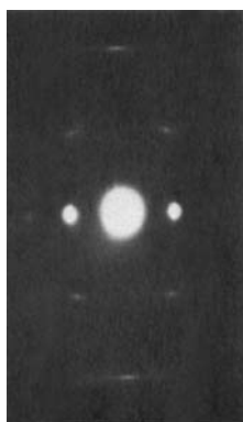
Fig.1 HEED pattern on a film with thickness <1000 Å
